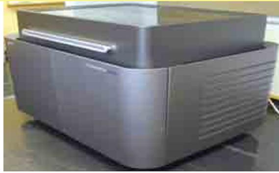
MDS has two 3D **Rapid Prototyping Printers** from Objet™: an Eden 260 and a Connex 350. These machines are used to build prototype parts for use as models or functional prototypes. Due to the additive nature of the build process, complex parts can be made that sometimes aren't possible with a traditional method of manufacture. Anatomical geometry taken from CT or MRI scans can be built as easily as a designed part. These machines allow us to build parts within hours.
