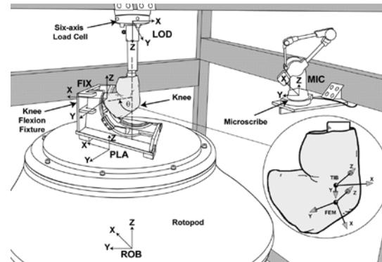
The UMS allows researchers to simulate loading conditions on cadaveric joints by using actuators to simulate muscle forces and simultaneously contact the joint with an external load. Applications of this type of testing are numerous and can be used to provide insights into orthopedics,
