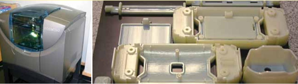
Since 2009, our engineers have used the Eden 260 **Rapid Prototyping System** to manufacture complex devices quickly.
